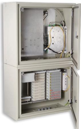
*The SI3000 ODU-XS is a small cabinet for FTTB or FTTN deployment scenarios. Compared to other FTTB solutions that require UTP cabling and several Ethernet switches, the SI3000 ODU-XS covers a multi-apartment building from a single location and requires only existing in-house copper cabling. Low investment costs and simple maintenance result in the overall lower operator's TCO.*
