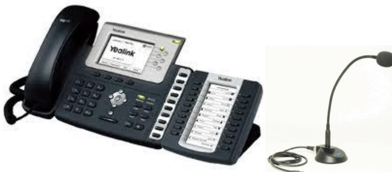
Figure 11: Basic dispatching terminal
