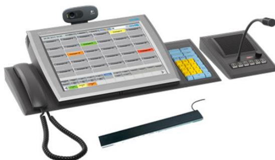
Figure 12: Multipurpose dispatcher terminal
